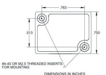
The A230 Air-In-line/Bubble Detector is one of our standard sensors for use with most tubing between 3 and 4 mm OD. It uses our proprietary digital non-invasive ultrasonic bubble sensing technology to accurately and reliably detect bubbles in a wide variety of fluids and tubing materials.
