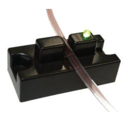
The A240 Air-In-line/Bubble Detector is one of our standard sensors for use with most tubing between 3 and 4 mm OD. It uses our proprietary digital non-invasive ultrasonic bubble sensing technology to accurately and reliably detect bubbles in a wide variety of fluids and tubing materials. The A240 uses a smaller area along the tube for easy and repeatable tube insertion.
